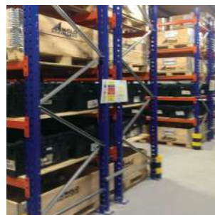
Adjustable Pallet Racking Well suited for order picking, but specialist equipment is necessary, e.g. dedicated traffic aisles, guidance systems rail or wire. Floor quality is critical, so a survey is required.
