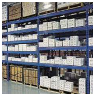
Random Location Best utilisation of space, any free storage location can be allocated to a SKU.
