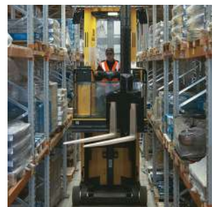
APR: Adjustable Pallet Racking – Automatic Storage and Retrieval System (AS/RS) Very high storage density, stacking heights 15 to 30m. Wind and building factors are critical, but planning restrictions and automation can reduce labour costs.
