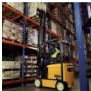
Fixed Location Every stock keeping unit (SKU) is assigned to a fixed storage location. Storage bays designed to handle maximum volume and load dimensions.
