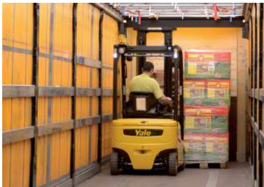
Compact trucks are able to work in lorries and containers.
